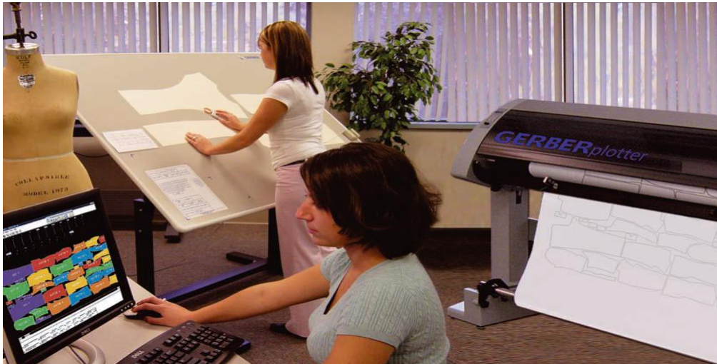
Figure 2: Digital Pattern and Marker Making CAD; Pattern Digitization and Pattern Prints Form Plotter (Source: Aldrich, 2009)
